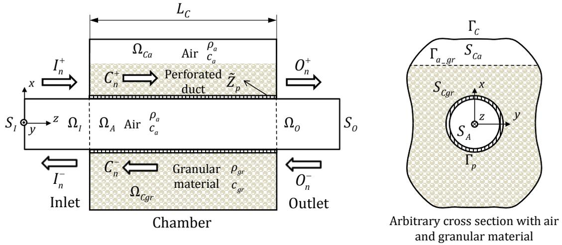
Figure 1. Scheme of silencer with granular material.
