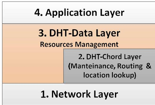
Fig.3. Main Functional Layers of a Peer-to-Peer Application
