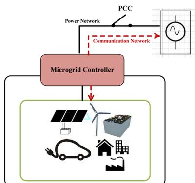
Fig. 1. Simplified scheme of a microgrid.
