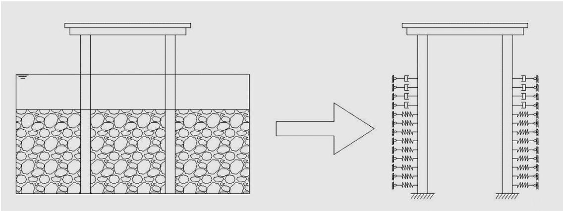
**Fig. 1.** Simplified Winkler beam model of the soil-structure system
