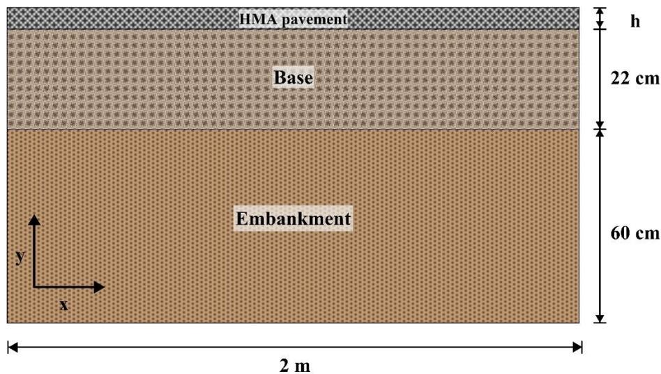
**Fig. 1.** Road section modelled in ANSYS
