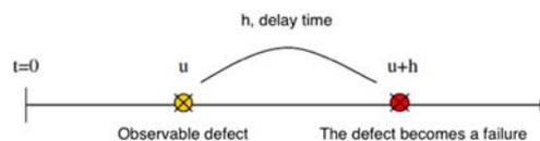
Figure 1. Time relationship between observable defect, failure and delay time
