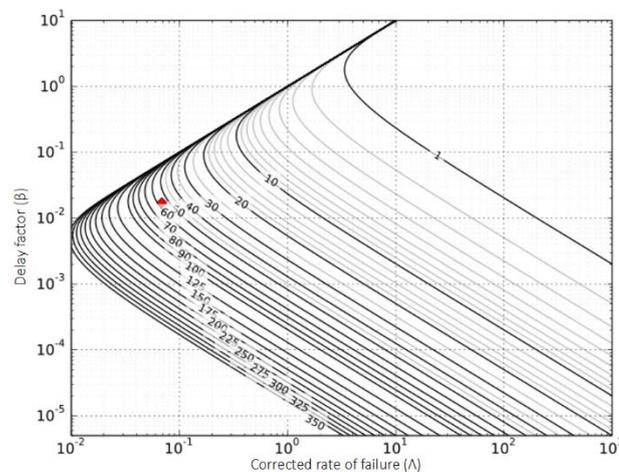
Figure 3. Optimum inspection period to obtain maximum savings per cycle based on  $\Lambda$  and  $\beta$  ( $T > t_i$ )
