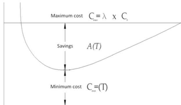
Figure 2. Costs per cycle based on the inspection period
